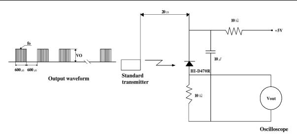
Fig.1 Standard transmitter
