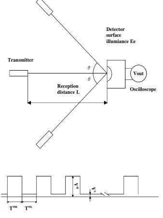
Fig.2 Standard optical test system
